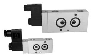
3/2-way solenoid valve, actuated by permanent signal for low temperature environment. Interface according to NAMUR-standard, with exhaust air recirculation (purge).
