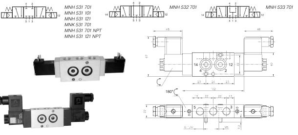
5/3-way solenoid valve with spring return to middle position. Interface according to NAMUR-standard.
