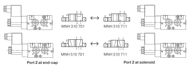
Single solenoid and single pilot valves are available with air spring or combined (air and mechanical spring) return.
