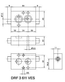
Type Function Port size Max. air flow Operating press. Weight DRN 3 611 VES 0,5 - 10 bar 0,42 kg 3-way valves Ø5mm 650 l/min ₩ **DRN 5 611 VES** 0,5 - 10 bar 0,42 kg \* 5-way valves Ø5mm 650 l/min **DRF 3 611 VES** 0,5 - 10 bar 3-way NAMUR-Flex Ø 5mm 650 l/min 0,42 kg
