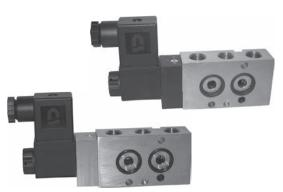
5/2-way solenoid valve, actuated by permanent signal. Interface according to 1/4" NAMUR-standard. Adding the **"Flex-Pack"**, converts the valve into a 3/2-way NAMUR-valve with exhaust-air recirculation ("purge").
