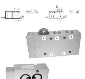
The **PN 411 721** is made for direct assemblage to an actuator with 1/4" NAMUR-interface. It offers a 1/4" NAMUR-interface towards the pilot-valve (use as sandwich plate) as well as ports G 1/4" for piped application. Delivery includes 2 screws, 2 O-rings.
