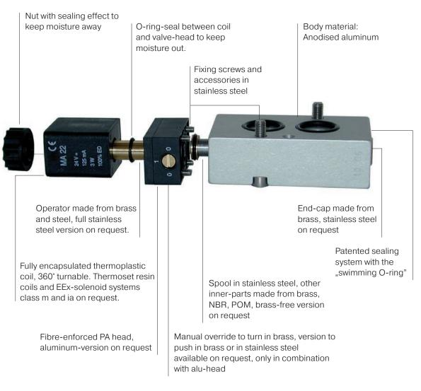
The special Hafner coil with covered yoke and additional seals between the coil and valve offers excellent protection in wet and humidity environment. Most Hafner solenoid valves offer IP65 as a standard and IP67 as an option.
