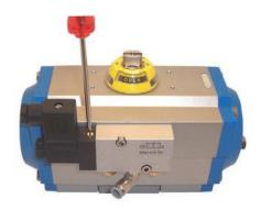
MNH 510 701 **H180** mounted on a double acting actuator. The pilot part is turned by 180°. The override is on the other side from the fittings. **Advantage:** Better accessibility
