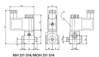
Direct acting 3/2-way solenoid valve equipped with spring return.
