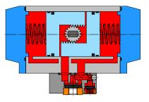
All 3-way Hafner NAMUR-valves ensure the exhaust air-recirculation! That applies also to our Hafner NAMUR-Flex valve (page 2.1.3).
