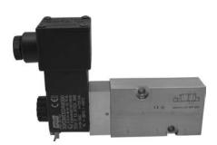
Material: Zone: Temperature range: Ignition protection type: Stainless steel, 316L 1, 2, 21, 22 -10°C ... +50°C Ex dm (encapsulatedflameproof with junction box) T5
