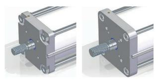
These kind of cylinders are mainly used for the automation of knife-gate-valves. Therefore the head of the cylinder has a mounting port pattern according to DIN 3358/ISO 5210 for direct mounting to knife-gatevalves.
