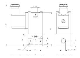
Direct acting 3/2-way and 2/2-way solenoid valve equipped with mechanical spring return. Orifice size: 3 mm, max. pressure: 7 bar.
