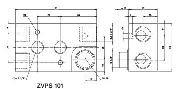
ZVPS 101 to be assembled onto an actuator with G 3/8" ports. Designed for an orifice size 10 mm in combination with e.g. MNH 510 101.
